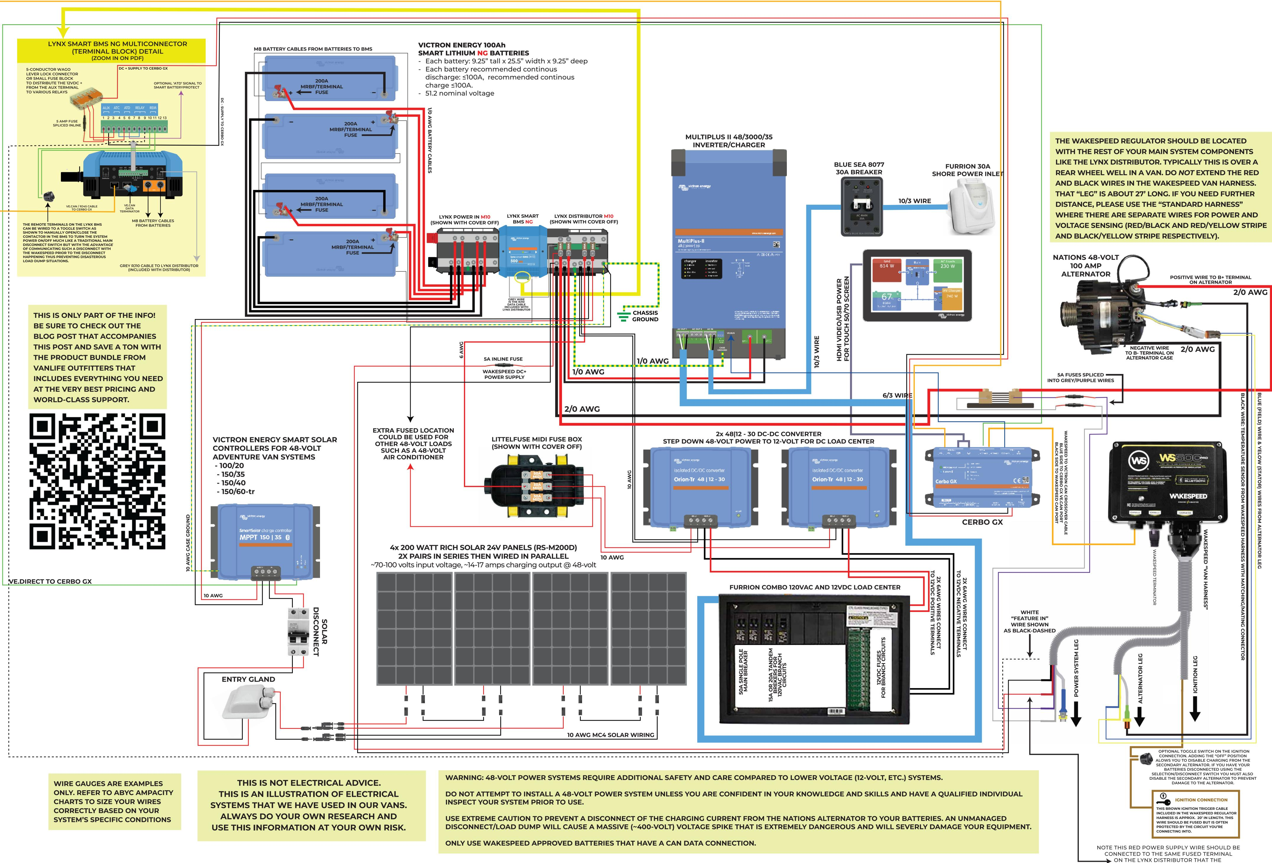
ALTERNATOR CHARGING OUTPUT IS CONNECTED TO AND CAN BE 48V.
